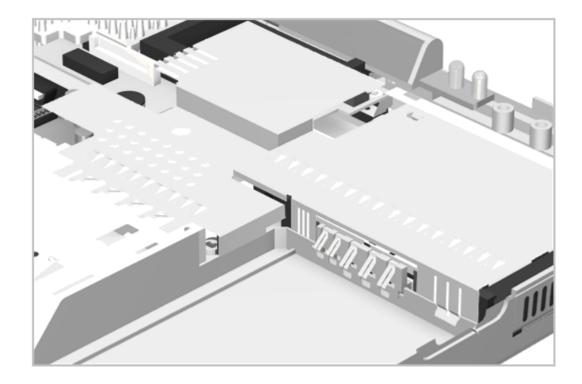
Figure 5-53. Placement of the EMI Shield
